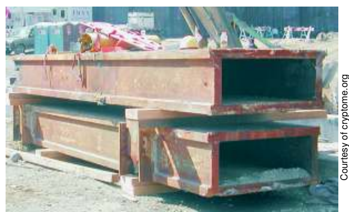
Figure 3-6 Core columns, sliced and ready to sell as scrap. This photo was taken at the WTC on October 3rd, 2001.
